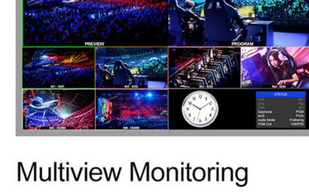
Multiview output make it easy to monitor 6 channels sources as well as PVW and PGM simultaneously on one display, besides, a clock and menu list are located in the lower right corner of the multiview.
