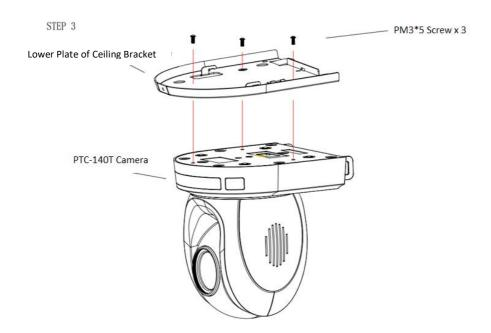
Step 4: Mount the PTC-140 Camera to the ceiling
