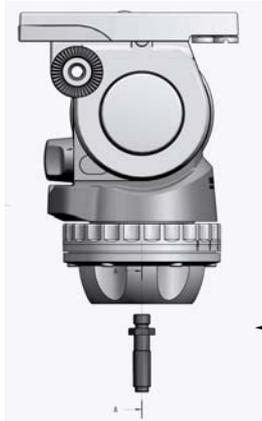
If you want to fit the FSB 4 onto a flat base, remove the threaded pin.
