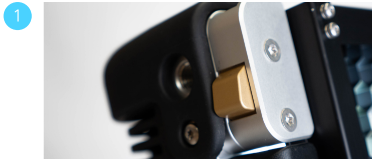
The filter rail slot has a unique locking mechanism that locks the initial filter in while allowing second filter to be inserted without unlocking.
