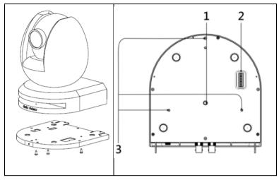
Figure 3. Screw 3 screws to ceiling Bracket A
