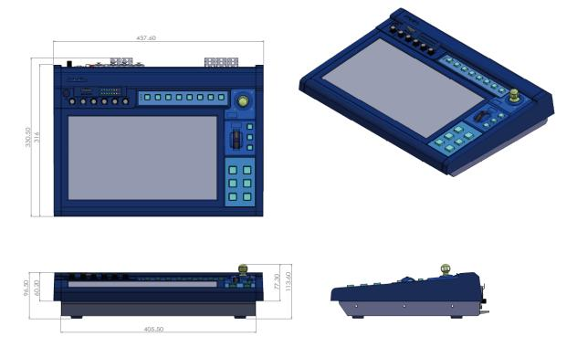
All measurements in millimeters (mm)
