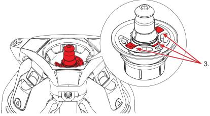
. Check that 3 lugs are correctly located in the Retaining Clip indents.
