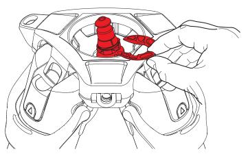
2. Holding the Bowl Connector in place with one hand, slide the Retaining Clip under 3 of the 4 positioning lugs on the Bowl Connector and snap into place.
