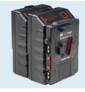
Use the PowerHub on the rear battery so that an accessory holder can be mounted to its face.
