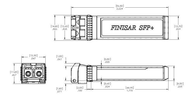
Figure 2. FTLX1471D3BCL Mechanical Dimensions.
