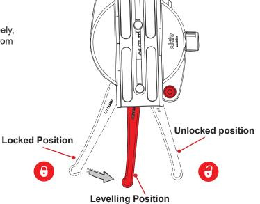
When head is fitted to the slider you may use the same procedure to fine adjust and check the level.
