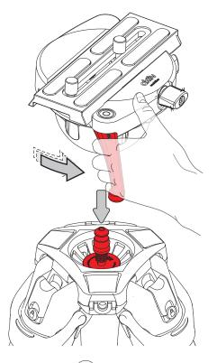
Hold the adaptor firmly with both hands. Pull the lever all the way back towards the level bubble.
