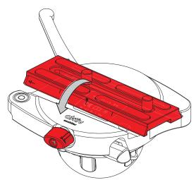
Place the camera plate with the slider fitted into the dovetail and lower into place.
