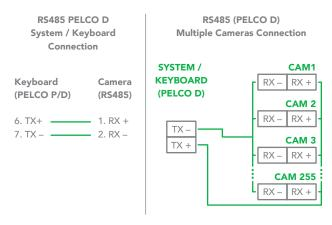
Connect the Camera's RS485+ and RS485 to RS485/TX+ and RS485/TX- on the control system/keyboard. The identity of the control system or equipment may be different; the corresponding relationship is as follows:
