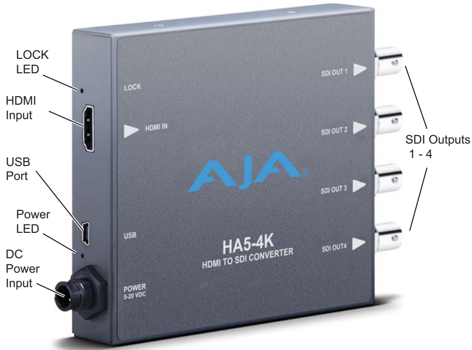
Figure 2. HA5-4K Converter Connections
