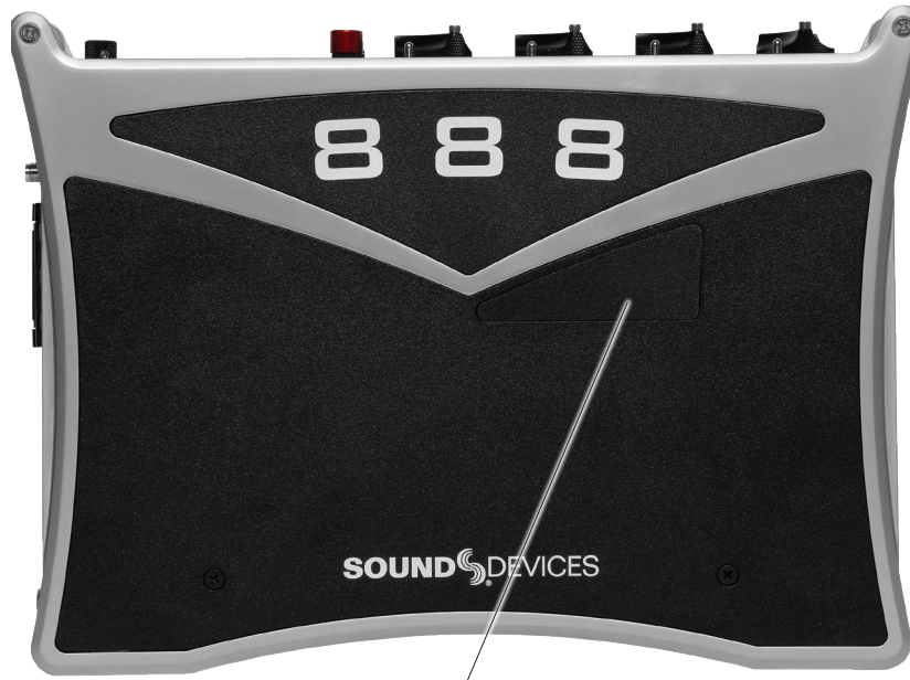
Test connector for manufacturing
